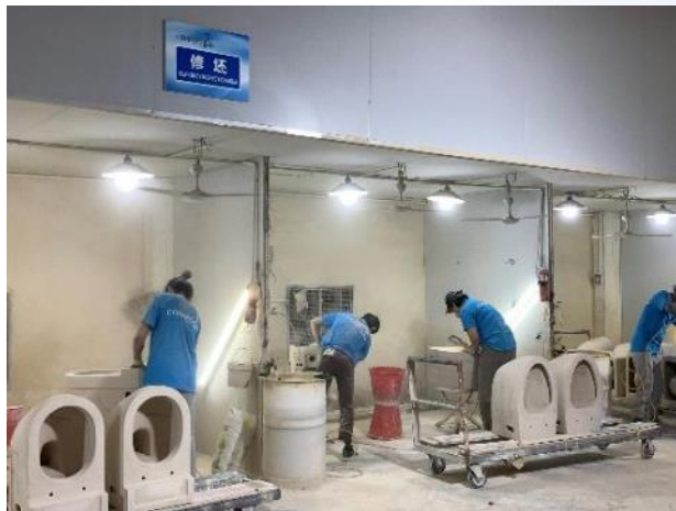
Air gun to clean the dusty on dry clay-body after Fettling and Inspection
