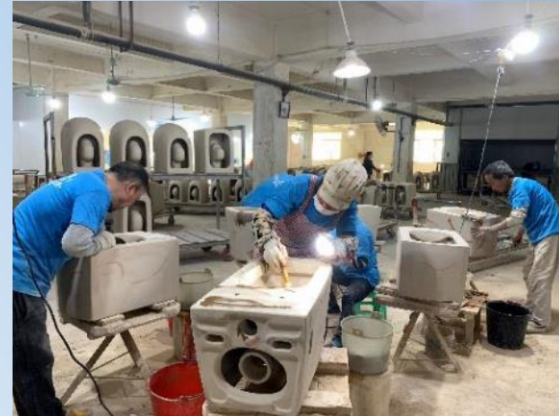
Air gun to clean the dusty on dry clay-body after Fettling and Inspection
